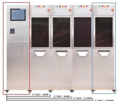
CMC-400 for 400 capsules/min, CMC-800 for 800 capsules/min and so on...
